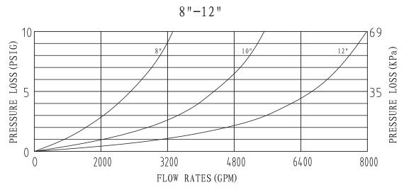
The above chart is based on clean water and ambient temperature.
